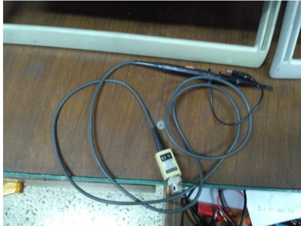
Gambar 4. 3 Kabel probe (Sumber : Laboratorium MEAS DTSP ITS)
