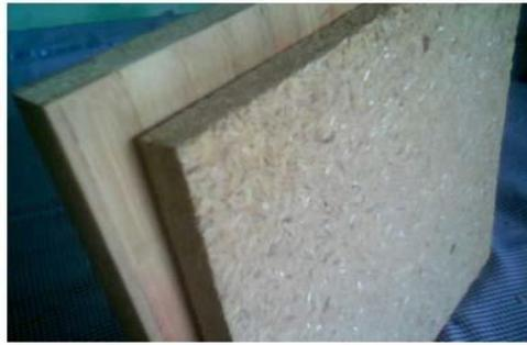
**Gambar 16** Coconut Fiber Cement Board
