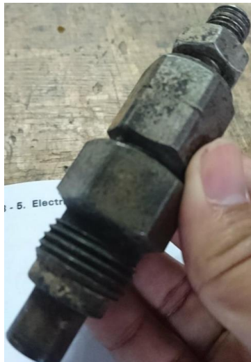
Figure 3.12 Injector of Mitsubishi 4D30
