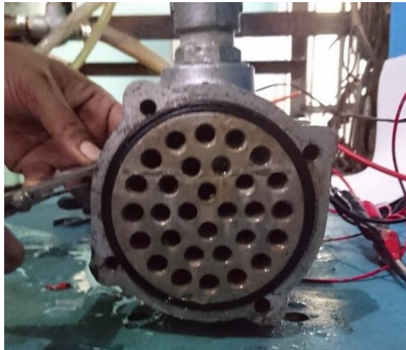
Figure 3.3 Cross sectional view of heat exchanger used in this experiment
