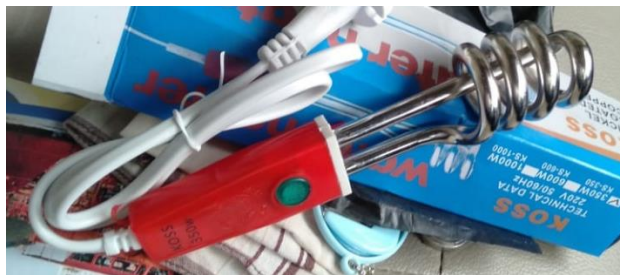
Figure 3.14 Electric heater for Spray Test Experiment
