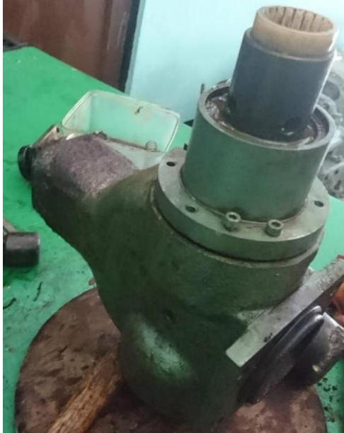
Figure 3.11 Water Brake Load Valve needs Bearing change
