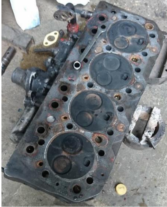
Figure 3.7 Checking the viability for drilling the cylinder head for pressure transducer
