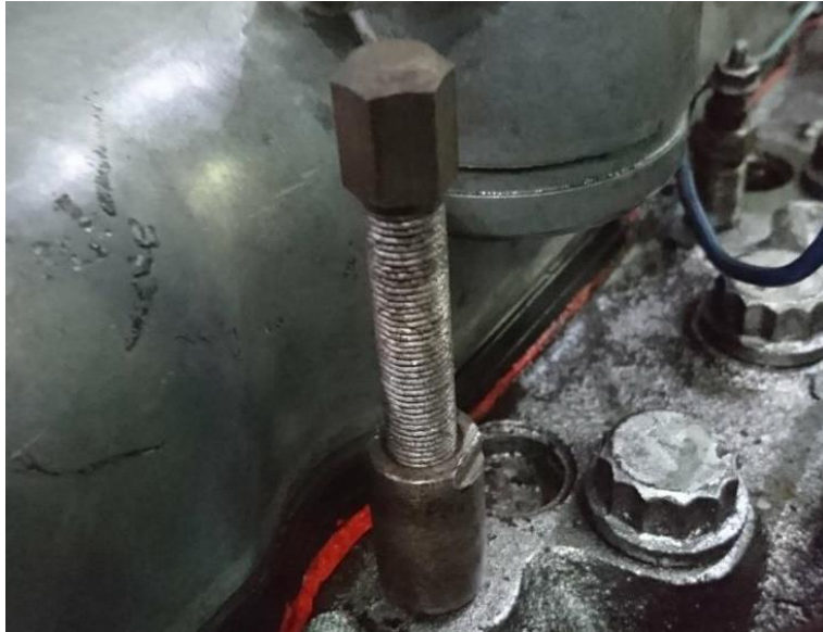
Figure 3.19 Connector for glow plug hole and Pressure transducer
