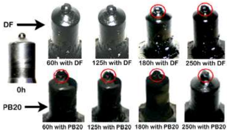
Figure 2.2 Photographic view on injector nozzle DF (Diesel Fuel) PB (Palm Biodiesel) [4]
