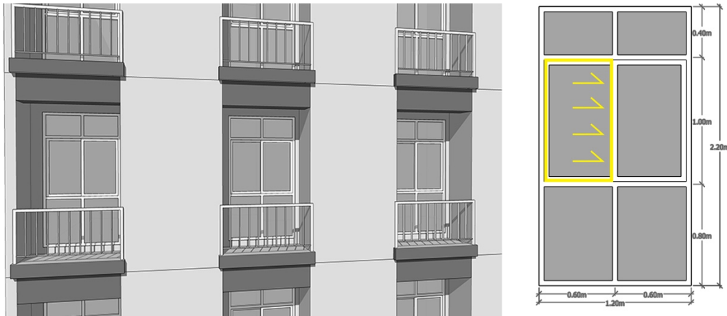
Figure 4.4 Illustration of Building Facade and Window Detail
