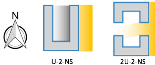
Figure 5.21 Illustration of Solar Radiation Penetrating the Courtyard due to Courtyard Opening
