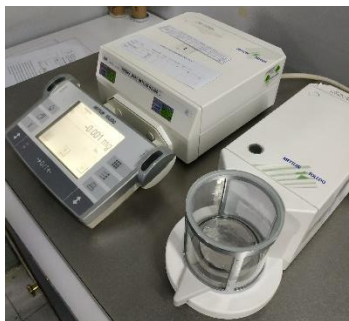
Gambar 3.8 Penimbangan filter sebelum sampling
