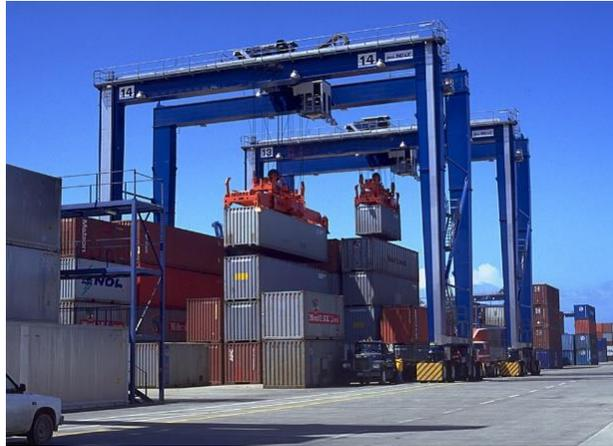
Gambar 2.3 *Rubber Tyred Gantry Crane*
