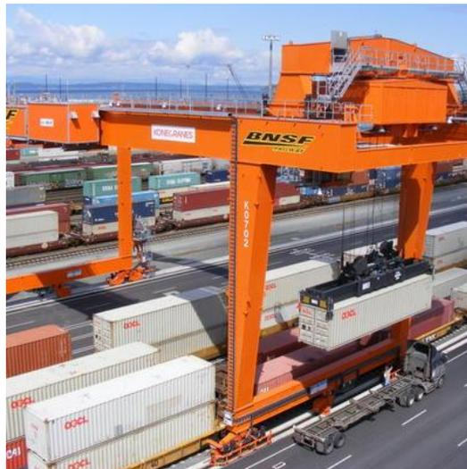
Gambar 2.2 Rail Mounted Gantry Crane
