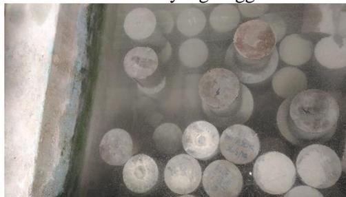
**Gambar 3. 8** Curing benda uji
