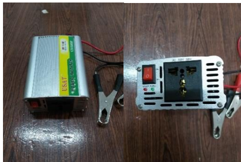
Gambar 3.10 Sine wave modified inverter.
