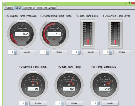
Gambar 4. 7 Windows Transfer Application Fuel Oil System
