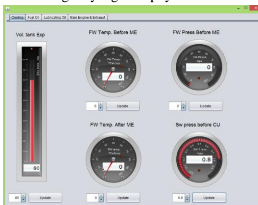
Gambar 4. 6 Windows Transfer Application Cooling System
