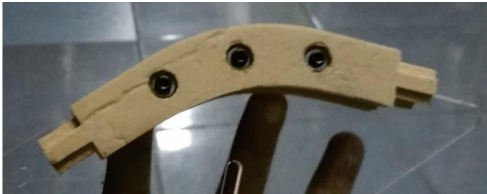
Gambar 4.68 Track melengkung diameter 70mm (Sumber: Data Pribadi)
