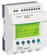
Gambar 3.2 Contoh PLC Compact [5]
