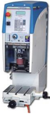
Gambar 3.1 Pad printing TAMPOPRINT [2]
