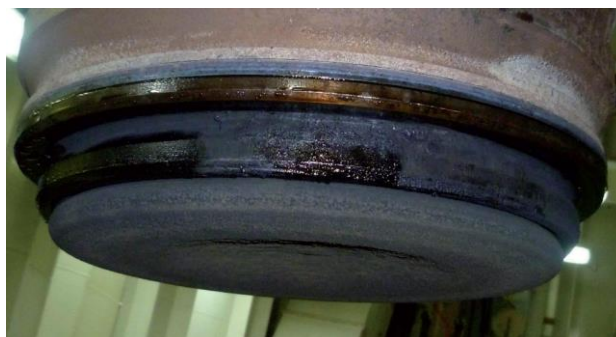
Figure 0.11 Exhaust valve spindle disk of MAN B&W Engine S60MC-C8.1
