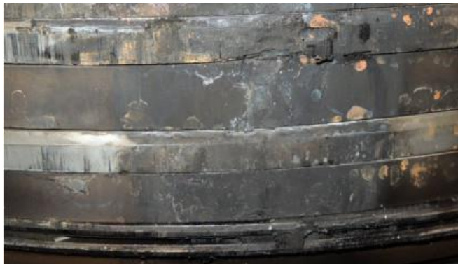
Figure 0.17 Stuck rings due to heavy carbon deposit
