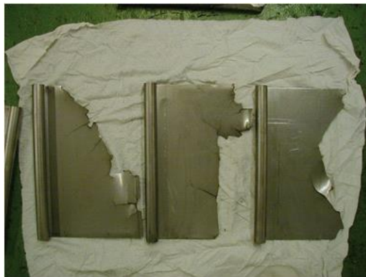
Figure 0.12 Broken flap valves
