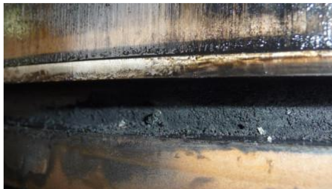
Figure 0.14 Clogged ring groove due to carbon deposits
