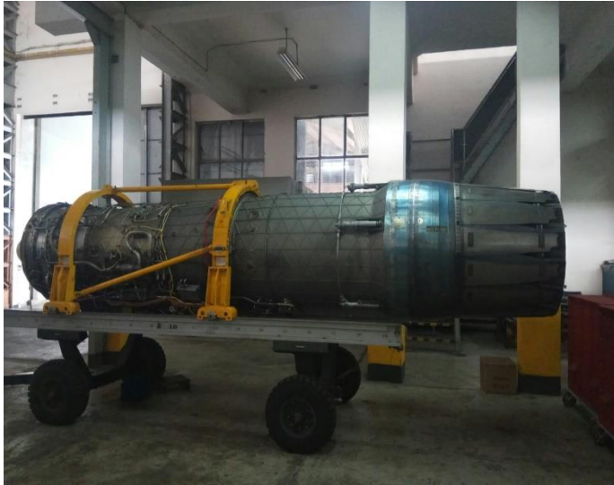
Gambar 3.1. Engine F100-PW-220 (F-16)
