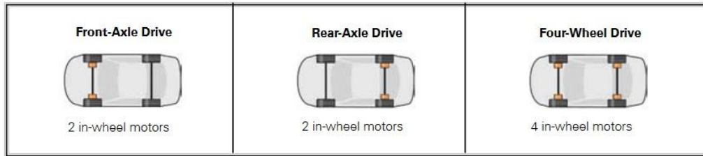
Gambar 2. 6 Jenis konfigurasi electric drive in the central . (volkswagen-newsroom.com, 2013)
