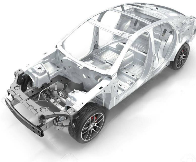
Gambar 4. 25 Unibody Chassis (ru.123rf.com)
