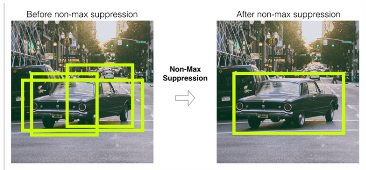
Gambar 3.33: Ilustrasi Proses Non-Max Suppression [[13]]
