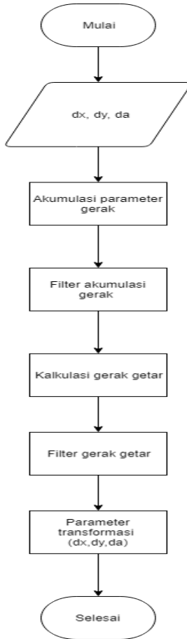
Gambar 3.16 Diagram alir pengolahan data tahap Motion compensation
