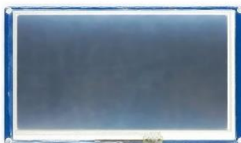
Gambar 2.15 Monitor Nextion tampak depan (Sumber : www.itead.cc )
