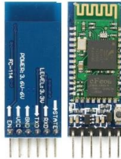
Gambar 2.12 Modul bluetooth HC-05 (Sumber : www.ram-e-shop.com )
