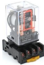
Gambar 2.11 Relay 8 pin (Sumber : www.amazon.com )
