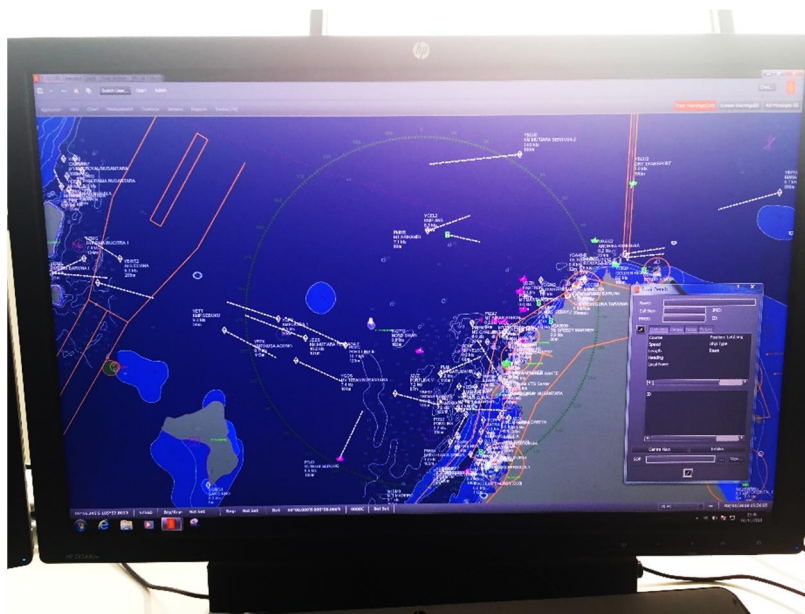
Figure 5.1 Actual Electronic Chart Display and Information System in Merak VTS
