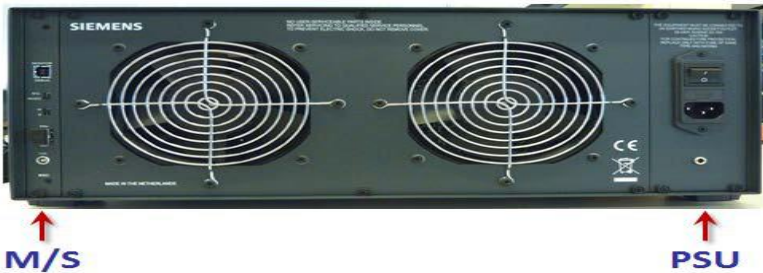
Gambar 3 LMS SCADAS Lab (Tampak Belakang) (LMS, 2016)
