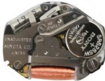
Gambar 2.7: Quartz Movement Sumber : Penulis, 2018
