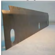
Gambar 21 Axial Seal Air heater
