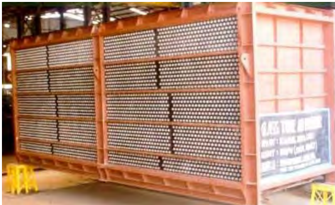
Gambar 9 Tubulat type Air heater (Sumber: Clean Boiler, 2014)
