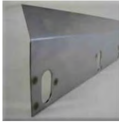
Gambar 19 Radial Seal Air heater
