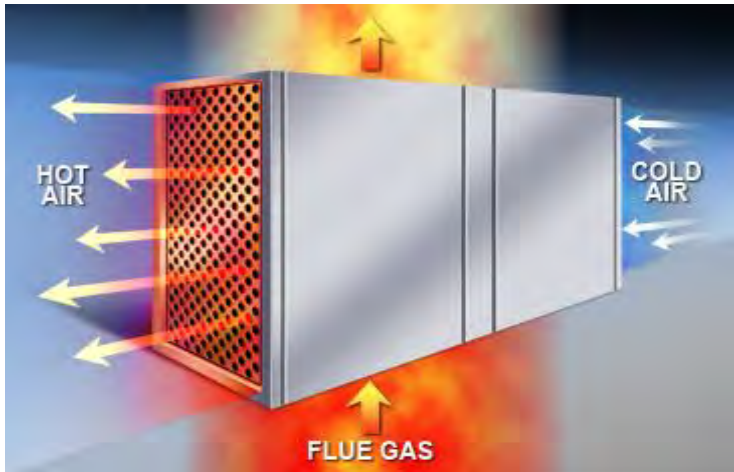
Gambar 8 Skema Arah Aliran Tubular Type (Sumber: Victory Energy, 2014)
