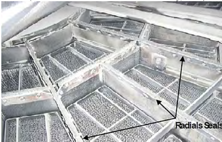
Gambar 20 Posisi Radial Seal
