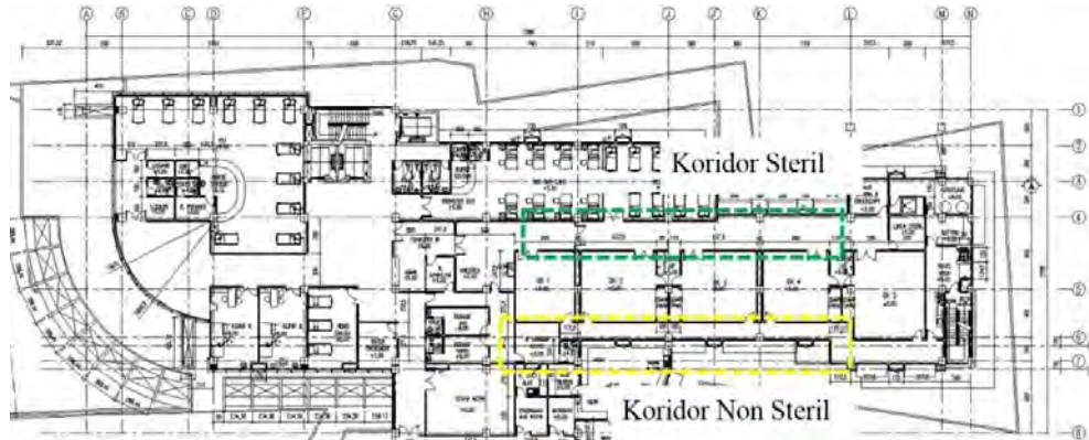
Gambar 2.11. Denah lantai 2 RSBS. (Sumber: DED RSBS)
