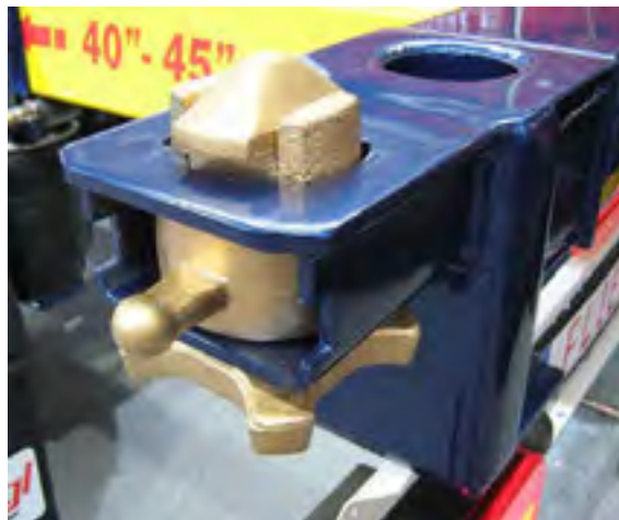
Gambar 4.29. Twistlock intermodal container (Sumber: Selbst, 2008)
