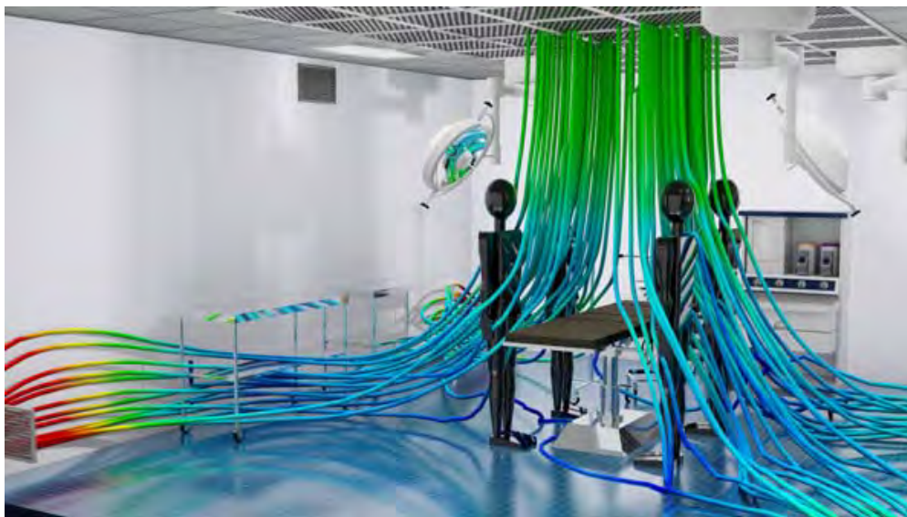
Gambar 4.35. Sistim laminar airflow (Sumber: http://machinedesign.com , 2016).
