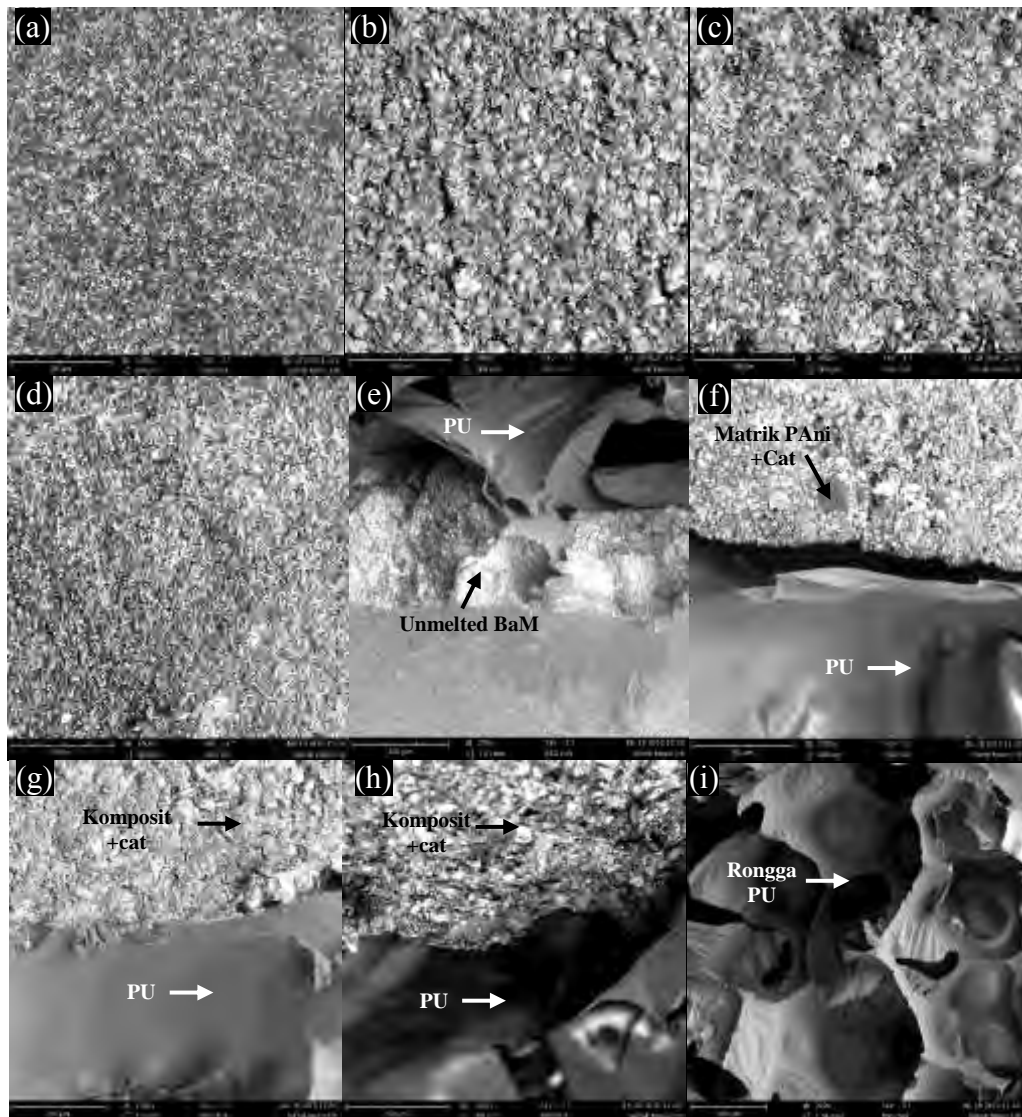
Gambar 4.13 Hasil SEM coating permukaan atas: (a) BaM/PAni 1000x, (b) BaM/PPy 1000x, dan (c) BaM/PET 1000x SEM coating penampang melintang: (d) BaM/PAni Dallenbach 1000x, (e) BaM/PAni Salibury 250x, (f) BaM/PAni Jaumann Layer 1000x, (g) BaM/PPy Jaumann Layer 1500x, (h) BaM/PET Jaumann Layer 1000x, dan (i) PU 200x
