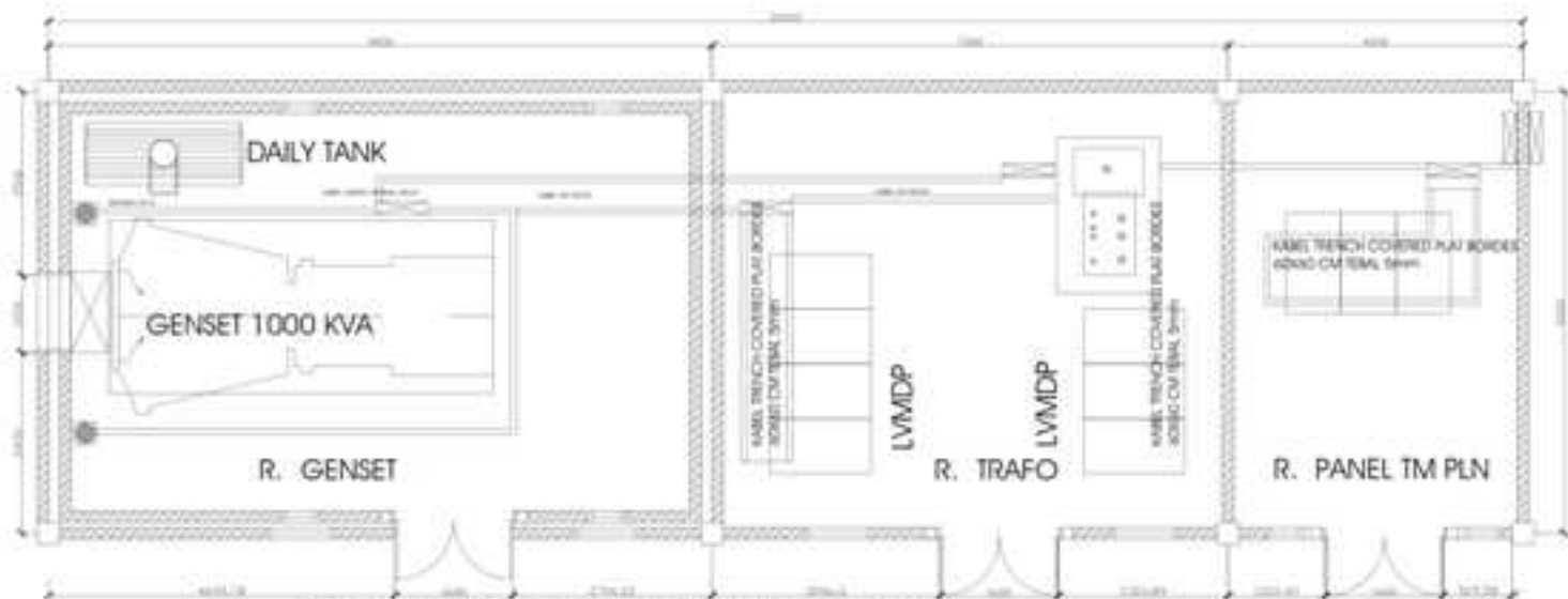
DENAH GENSET, TRAFU, PLN SKALA 1:50
