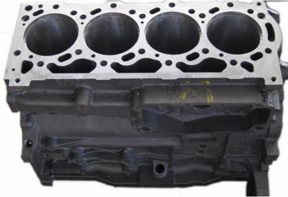
**Gambar 2.14 Blok mesin (rizal, 2012)**
