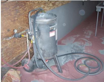
**Gambar 3. 3** Alat *Sand Blasting*
