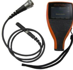
**Gambar 3. 2** DFT (*Dry Film Thickness*)
