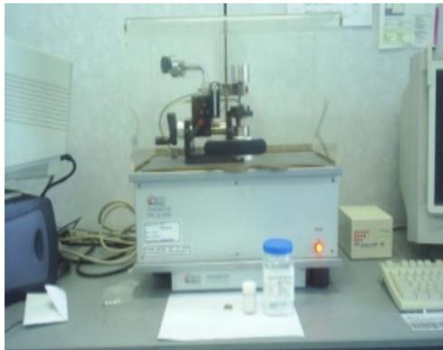
**Gambar 3. 6** Alat Uji Aus *Pin on Disk*
