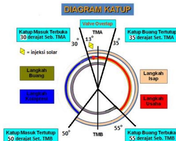
Gambar 2.18 Diagram katup motor diesel
