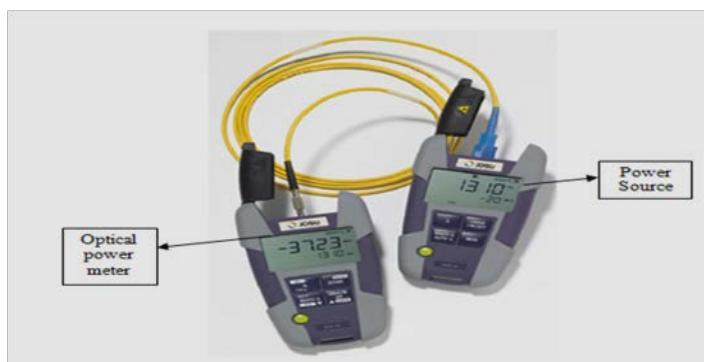
**Gambar 2.10.** Optical power meter dan power source
