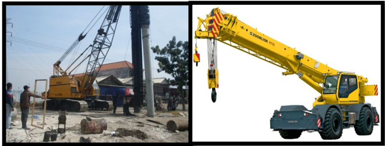
Gambar 2.9 Crane Hammer, Crane Service dan Crane Erection
