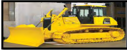
Gambar 4.4 : Bulldozer Komatsu D155AX – 5 SL
