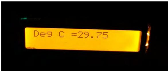
**Gambar 3.8** Indikator LCD 16x2
