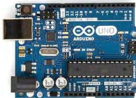
**Gambar 2.2** Microcontroller Arduino Uno
