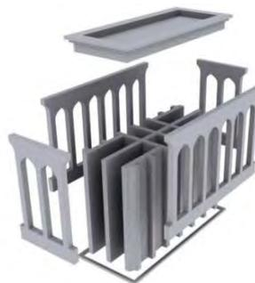
Gambar 2.53 3D model *windcatcher with different canals* (Zarandi, 2009)
