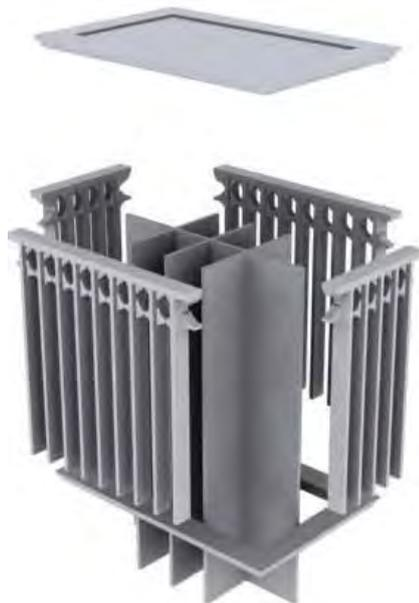
Gambar 2.51 3D model *windcatcher with equal canals* (Zarandi, 2009)
