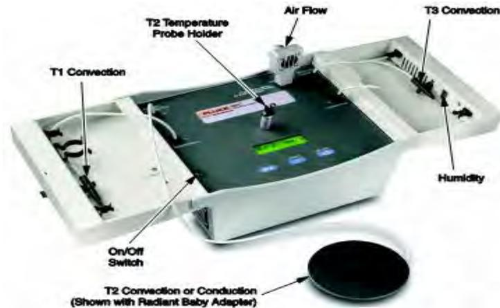
*Gambar 2.2 Incubator Analyzer*
