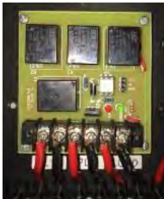
Gambar 3.10 Auto Switching Driver Relay
