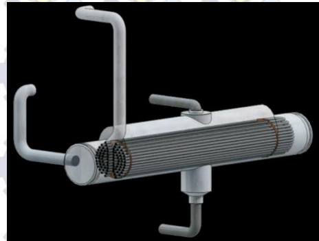
Gambar 2.17. Brine Heater (sumber : PPT Desalination Plant PT. PJB UP Gresik)
