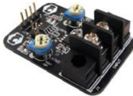
Gambar 2.3 Sensor Arus ACS 712
