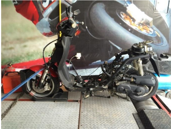
Gambar 3.4 Set up Waterbrake Dynamometer Torsi Motor listrik
