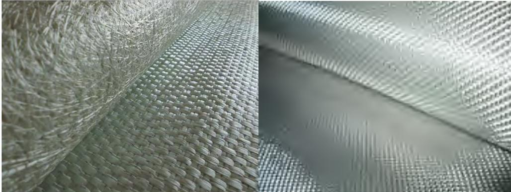
**Gambar 3.4** (a) Serat fiber Combo mat (b) serat fiber tipe *cloth*
