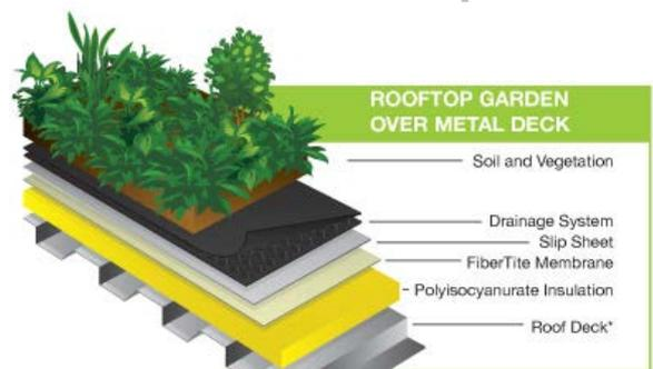
Gambar V. 12 Diagram green roof
