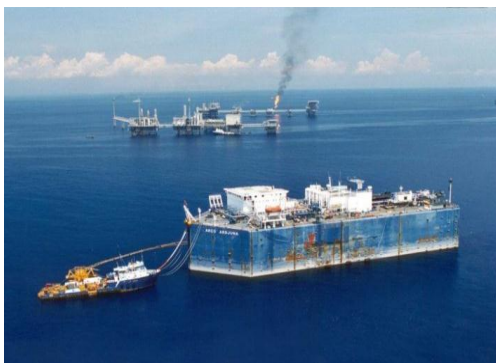
Gambar 1. FSO Arco Ardjuna tertambat SPM (Sumber: PT. Citra Mas, 2014)
