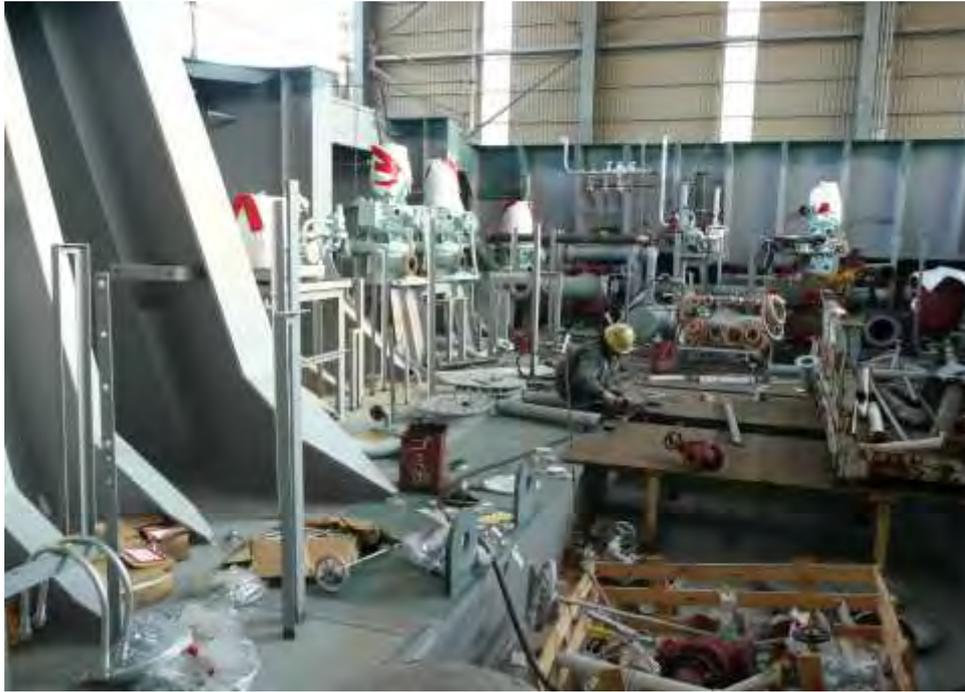
**Foto full outfitting block system (FOBS) setelah proses block blasting dan painting.**
