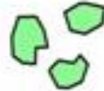
Angular (mechanical disintegration, carbonyl (Ni))
