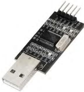
**Gambar 2.10** Modul USB to RS232 TTL
