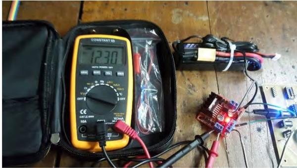
**Gambar 4.4** Rangkaian *Driver* L298 Modul *Solenoid*
