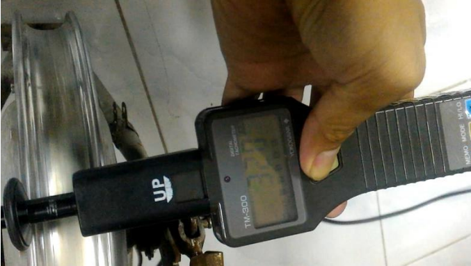
Gambar 4.24 Measurement of RPM motor with tachometer
