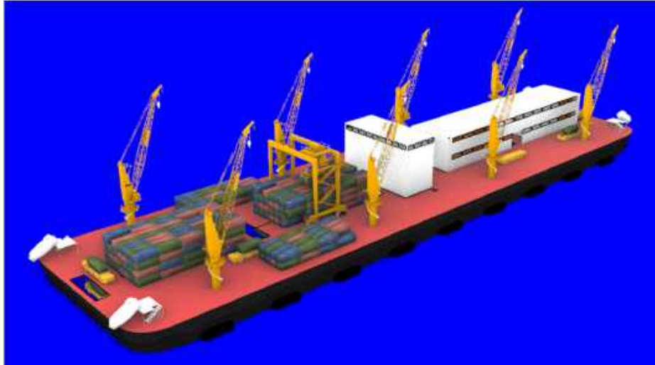
Gambar 4.33 Gambar 3D Floating Supply Mobile Offshore Base
