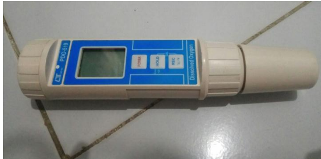
Gambar 3.14 Dissolved oxygen meter jenis Lutron 519
