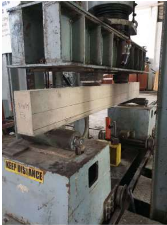
Gambar 4.6 Set-up pengujian pre-crack
