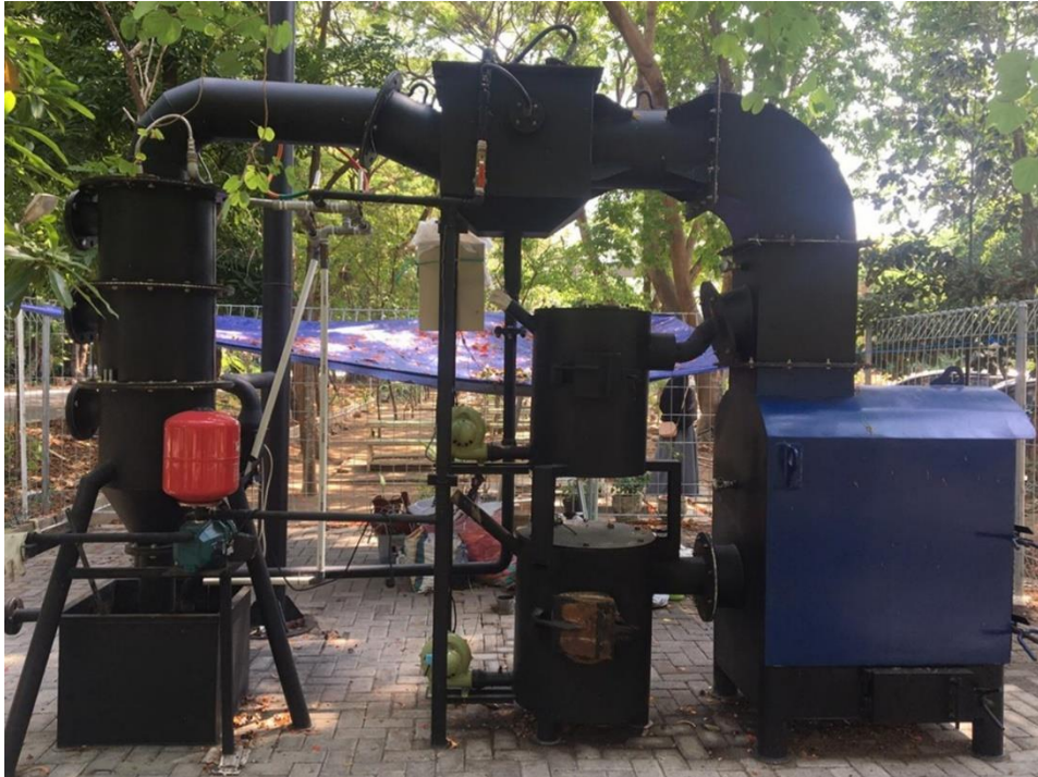
Reaktor wet scrubber
