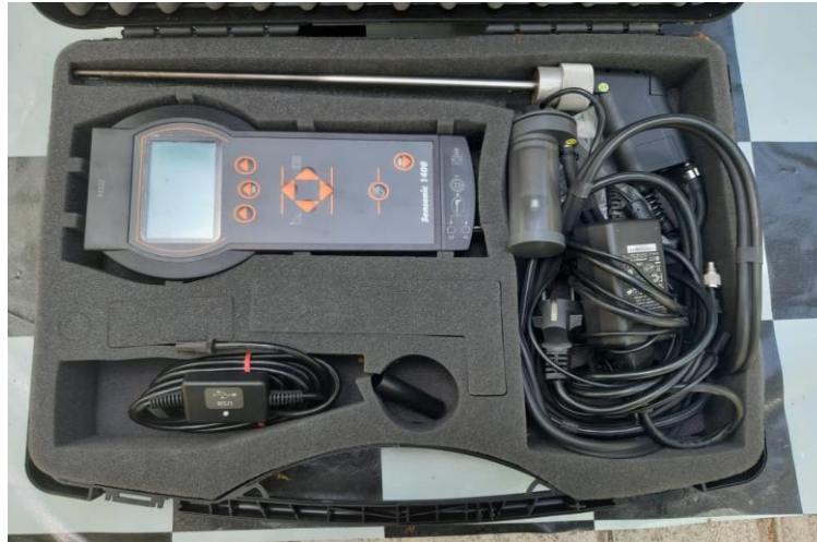
Gas analyzer sensonic type 1400
