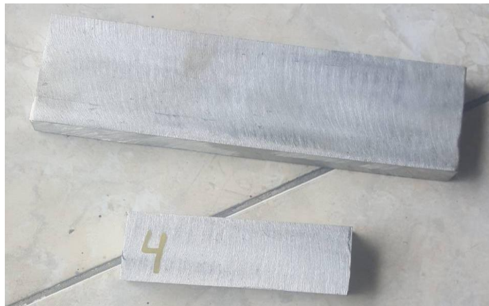
Gambar III.6 Contoh tanggem dudukan (atas) dan tanggem start/stop
