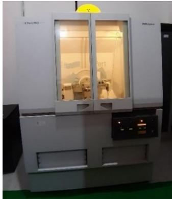
**Gambar 3.3** Alat *X-Ray Diffraction* (XRD)
