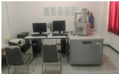
**Gambar 3. 4** Alat *Scanning Electron Microscope* (SEM)
